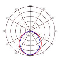
e beam angle(50%):109.5(DEG) C90 Plane beam angle(50%):99.1(DEG)
